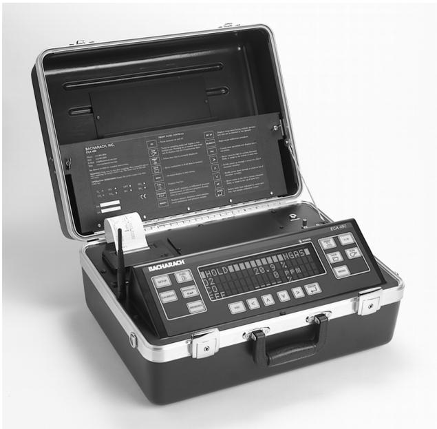
**Figure 5-14. Combustion Efficiency & Environmental Analyzer.** Photo courtesy of Bacharach Instrument Company
