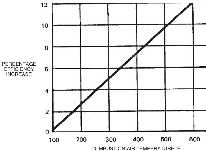
Figure 10-4. Efficiency Increase with Pre-Heated Air
