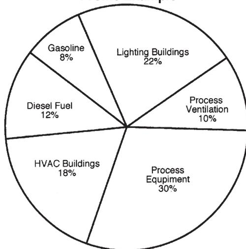
Figure 2-7. Energy Profile by Function
