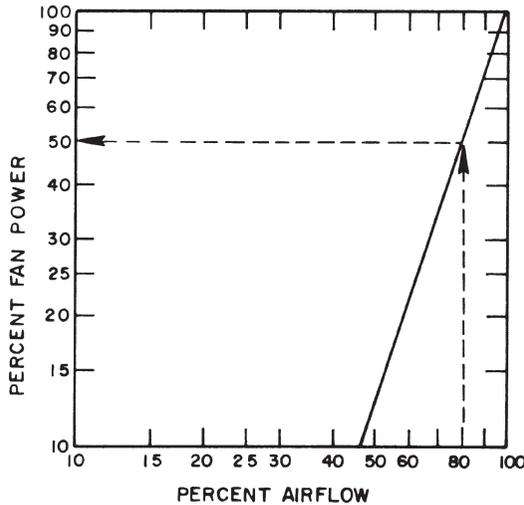
Figure 8-2. Decrease in Horsepower Accomplished By Reducing Fan Speed (Based on Laws of Fan Performance). (Source: NBS Handbook 115 Supplement 1)
