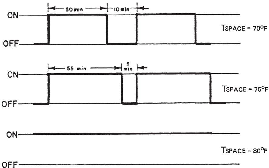
Figure 7-7. Temperature Compensated Duty Cycling
