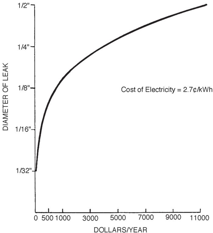
**Figure 10-7. Cost of Air Leaks at 100 PSI (Source: *Instructions For Energy Auditors, Volume II*)**
