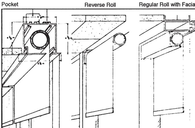
Figure 6-24. Motorized Shade System
