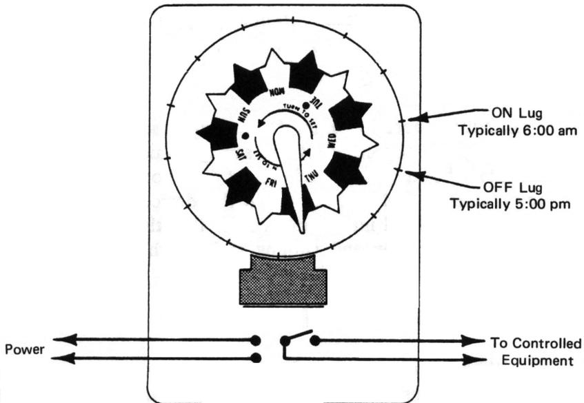
Figure 7-6. Mechanical Timeclock
