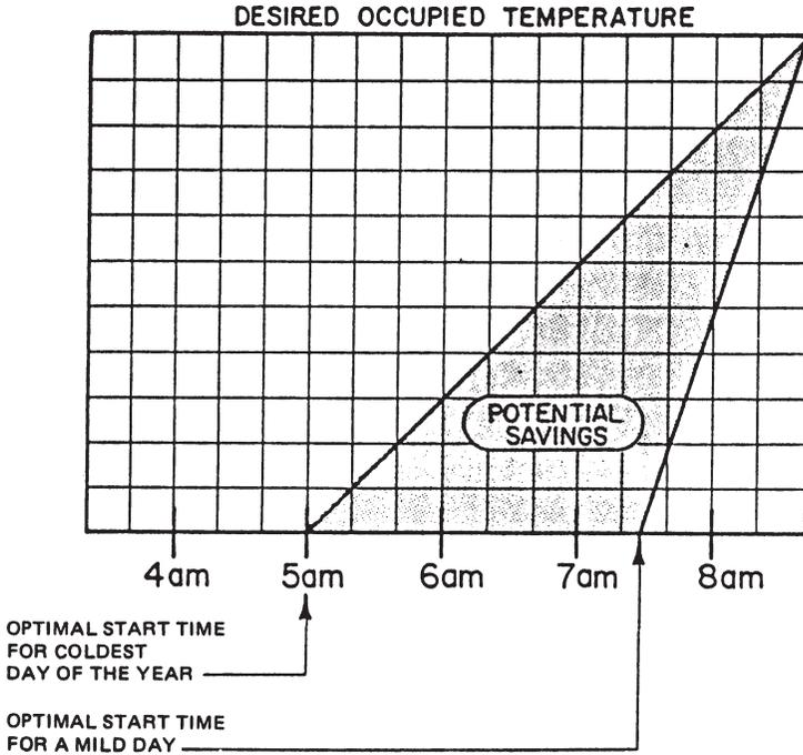
Figure 7-10. Typical Variation in Building Warm-Up Times
