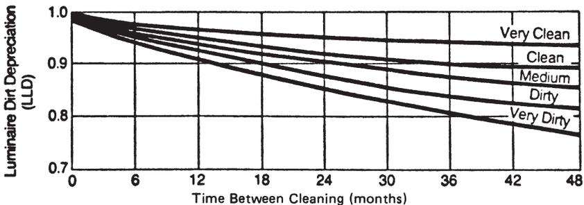
Figure 7-4. Effect of Dirt Build-Up on Dust-proof Luminaires for Various Atmospheric Conditions
