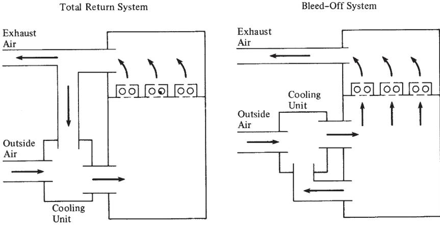
Figure 8-12. Recovery from Lighting Fixtures
