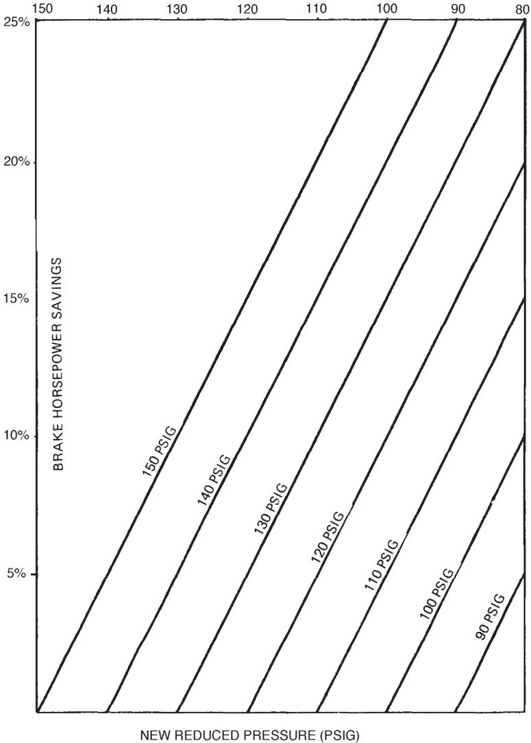
Figure 10-8. Savings with Reduction in Pressure (Source: *Instructions for Energy Auditors, Volume I*)
