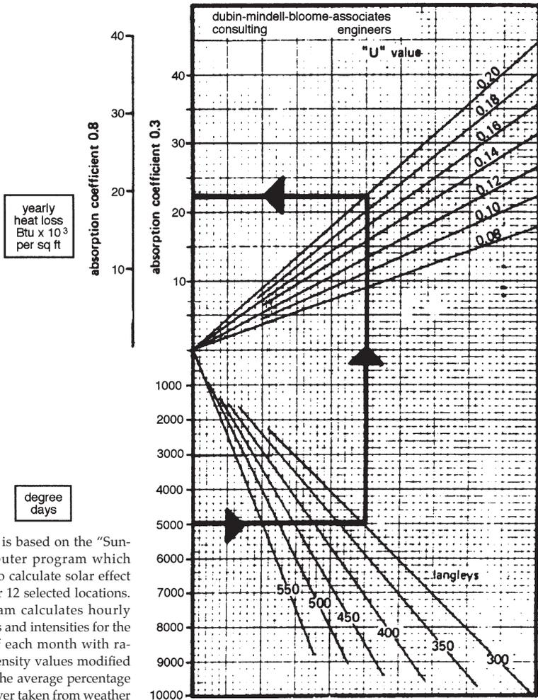
This figure is based on the "Sunset" Computer program which was used to calculate solar effect on roofs for 12 selected locations. The program calculates hourly solar angles and intensities for the 21st day of each month with radiation intensity values modified hourly by the average percentage of cloud cover taken from weather records. Heat losses are based on a 68F indoor temperature.
