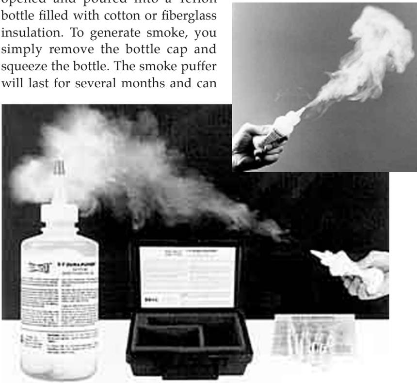
Figure 5-4. Chemical smoke kit. Photo courtesy of E. Vernon Hill, Incorporated.
