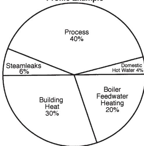
Figure 2-8. Steam Profile by Function
