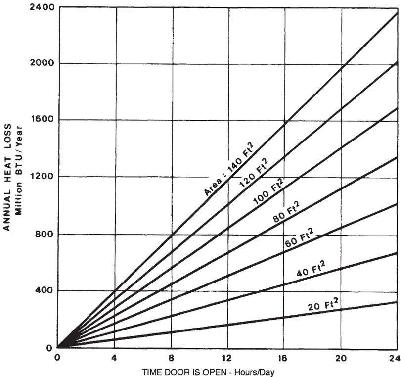
Figure 6-3. Annual Heat Loss from Doors. (Source: Georgia Tech Experiment Station)
