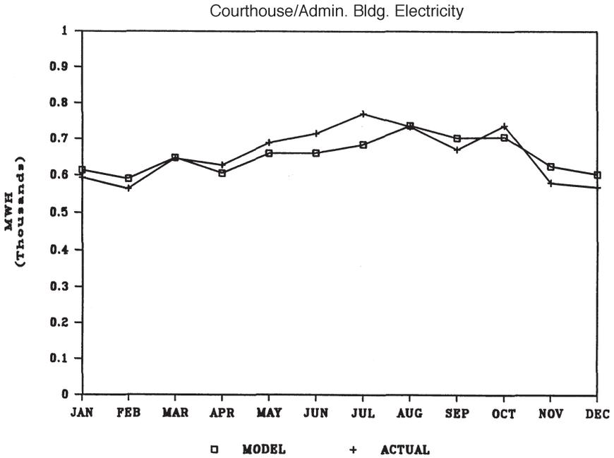
Fig. 16-2. Comparison of model and actual annual electrical use profile.
