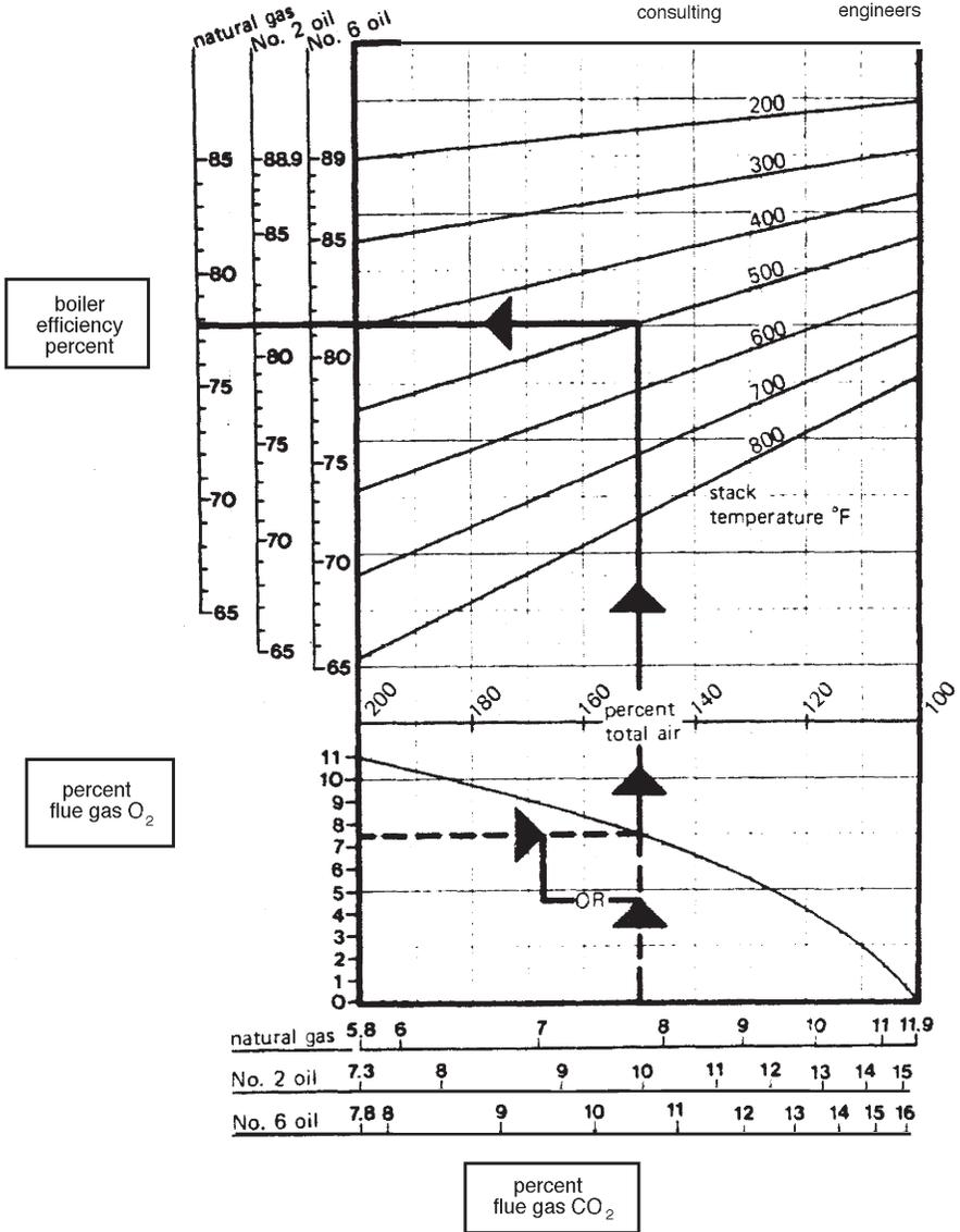
Figure 10-3. Effect of Flue Gas Composition and Temperature on Boiler Efficiency (Source: *Guidelines For Saving Energy in Existing Buildings—Engineers, Architects and Operators Manual, ECM-21*)
