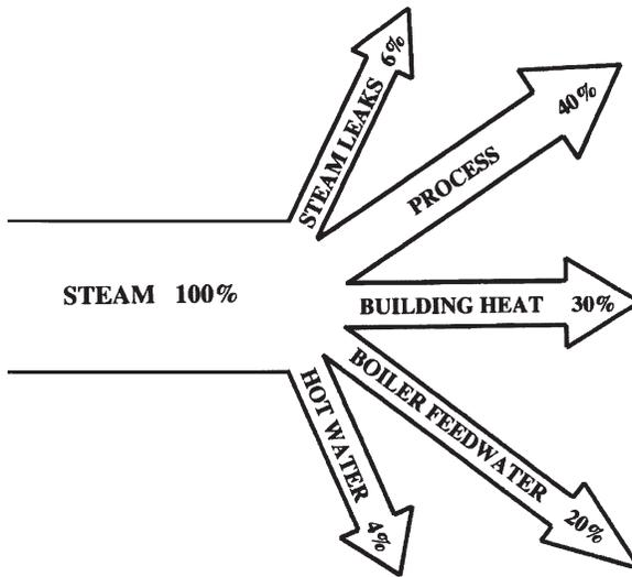
**Figure 2-9. Steam Distribution Nodal Diagram Example**
