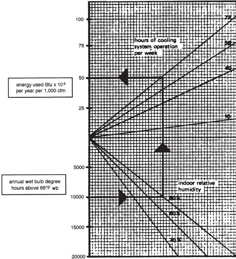
**Figure 6-7. Yearly Energy Used Per 1,000 CFM to Maintain Various Humidity Conditions (Source: Guidelines For Saving Energy in Existing Buildings—Building Owners and Operators Manual, ECM-1)**
