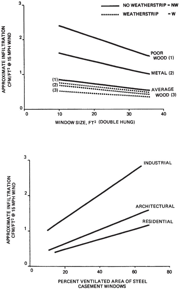
Figure 6-5. Infiltration through Windows and Doors—Winter. (Source: Instructions For Energy Auditors, Vol. II)
