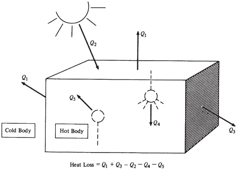
Figure 6-2. Heat Loss of a Building
