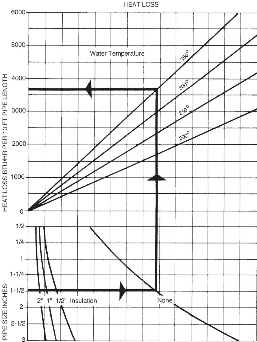
Figure 10-10. Pipe Heat Losses
