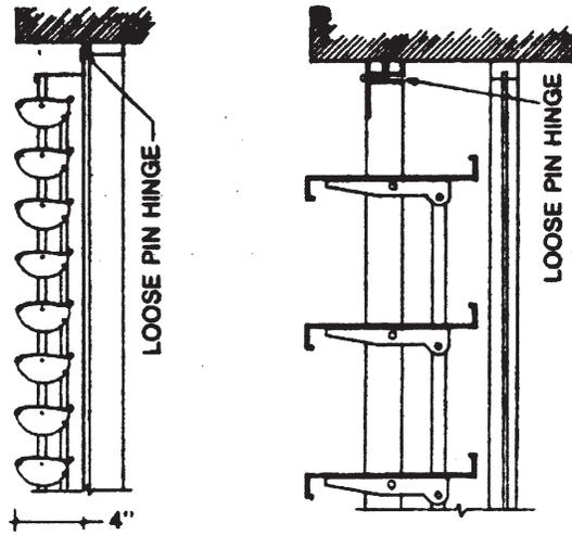
**Figure 6-25. Mounting of External Louvers**
