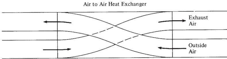
AIR-TO-AIR HEAT PIPES AND EXCHANGERS
