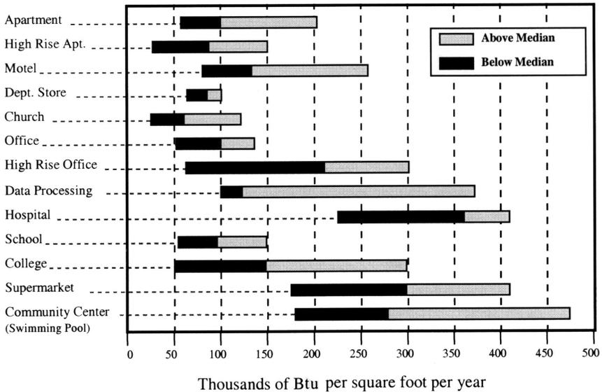
Figure 2-2. Energy Use Index by Building Type
