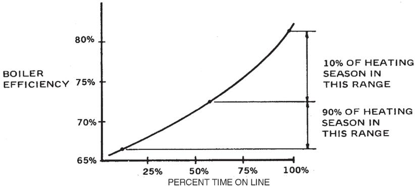
Figure 10-5. Effects of Boiler Cycling
