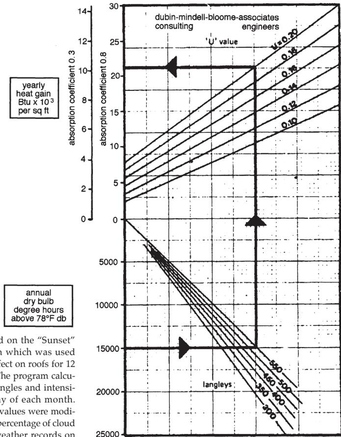
This figure is based on the "Sunset" Computer program which was used to calculate solar effect on roofs for 12 selected locations. The program calculates hourly solar angles and intensities for the 21st day of each month. Radiation intensity values were modified by the average percentage of cloud cover taken from weather records on an hourly basis. Heat gains are based on a 78F indoor temperature.
