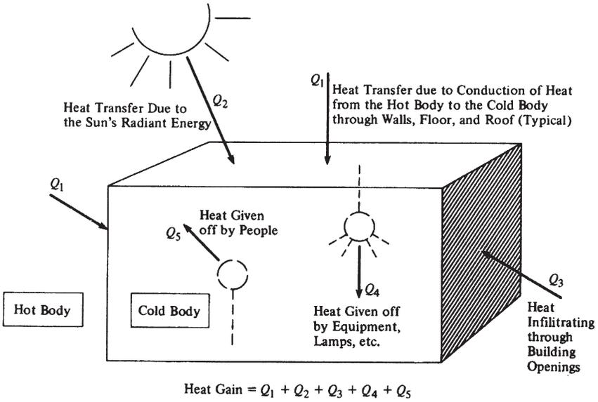
Figure 6-1. Heat Gain of a Building
